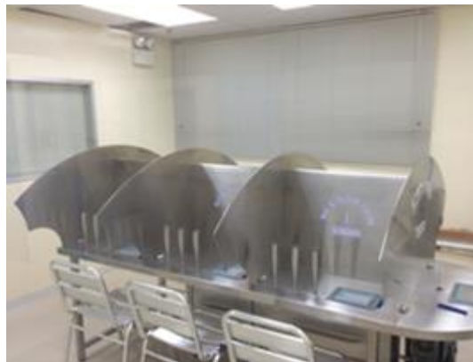
Figure 3: Olfactory Laboratory with Scentroid™ SS600 Olfactometer
